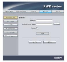
This screen lets you make settings for display and playback of still image and video files stored on a Web/HTTP server. A maximum of 1,000 files can be downloaded with Store Local. Each file can be no larger than 2 GB in size.
